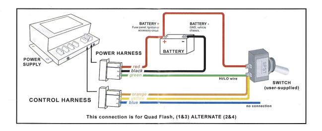
**IV. Wiring Control Harness.** Combination of different wires (**ORANGE**, **YELLOW**, **BLUE**) allow for different flash patterns; (see table). The **GREEN** wire from Power Harness enables High/Low Power function; (when off, it's at High Power, and when on, it's at Low Power. The remaining unused wires may be removed or left in place for future alterations. For FP#5, High Power function enables Mega Flash, and Low Power function enables Quintuple Flash.
