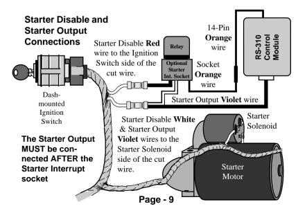
Connect the 14-pin connector's Orange wire to the Orange wire of the starter interrupt relay socket. Then make the connections which interrupt the vehicle's starter circuit- the starter wire must be located and cut. Cutting the vehicle's starter wire will result in two sides- the "ignition switch" side and the "starter solenoid" side. It is recommended that this connection be done as close to the ignition switch as possible. Use a Digital Multimeter (DMM) to find the correct wire.
