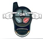
• THE HORN WILL SOUND AND THE DOORS WILL LOCK OR UNLOCK DEPENDING WHICH BUTTON IS PRESSED.
