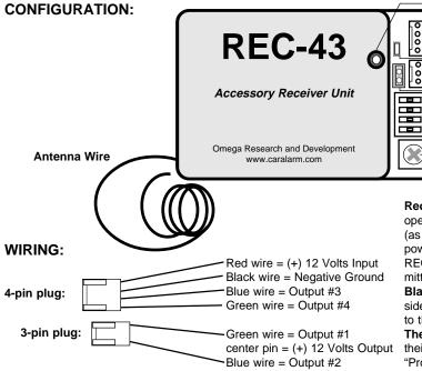
**Opening on top of module:** Provides access to the Transmitter Programming Switch
