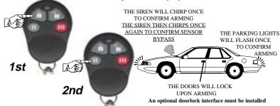
Remote Sensor Bypass allows the option of "turning off" the sensor any- time the system is armed using the transmitter. When the sensor is bypassed, only the sensor zone is bypassed and all other protected zones will remain fully operational and vigilant. The sensor zone will reset to its normal operation the next time the system arms.
