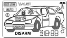
transceiver will unlock the doors <u>unless</u> the system is activated and sounding.
