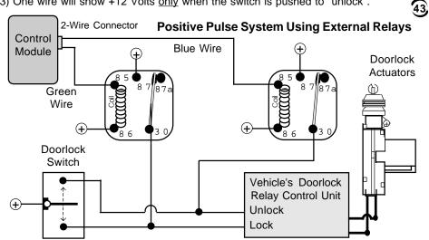
Warning: The Positive pulse system can be confused with the 5-wire Reversing Polarity system. This is because both systems show +12 Volt pulses on the "Lock" and "Unlock" wires when the vehicle's switch is pressed respectively. It is critical to identify which system is present, since if +12 Volts is pulsed into a Reversing Polarity system, which rests at ground, a direct short circuit will occur.
