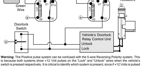
is because both systems show +12 Volt pulses on the "Lock" and "Unlock" wires when the vehicle's switch is pressed respectively. It is critical to identify which system is present, since if +12 Volts is pulsed into a Reversing Polarity system, which rests at ground, a direct short circuit will occur.
