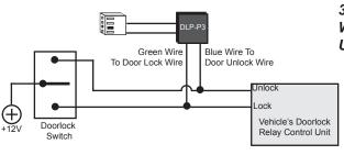
3 Wire Negative Doorlocks With All Unlock Function Using Optional DLP-P3
