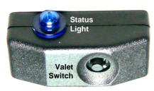
vehicle. If the optional Echo 2-way controller is used, the Status Light and Valet Switch are within a long-range receiver module, typically mounted to the windshield or other glass. The Status Light may be either blue or red; included with your K-9 system is a blue light (red is available optionally), and
