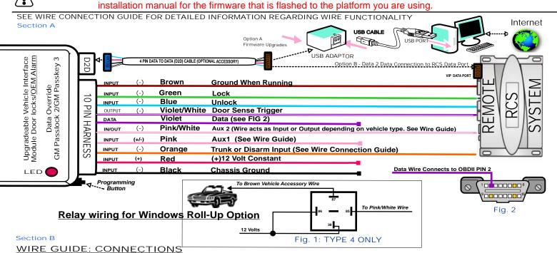
10 PIN HARNESS → D2D = Optional use of 4 Pin Data to Data (D2D) cable will replace the analogue wire (w2w) connection
