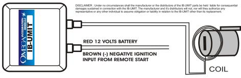
Locate the coil around the ignition cylinder
