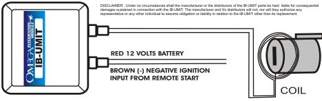
Locate the coil around the ignition cylinder
