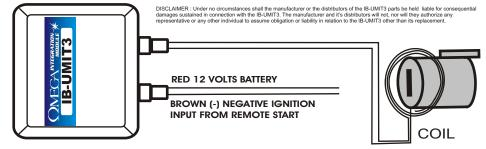
Locate the coil around the ignition cylinder NOTE: 2 OR 3 TURNS OF LOOP IS REQUIRED
