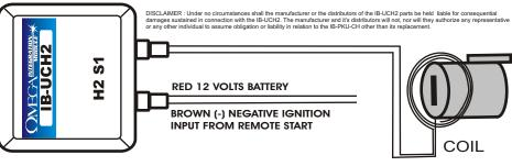
Locate the coil around the ignition cylinder
