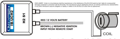
Locate the coil around the ignition cylinder
