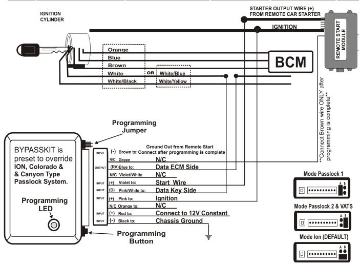
INSTALLATION NOTES: \*Saturn ION, GMC Canyon & Chevy Colorado etc do not have starter wires. \*\*This self learning kit will not function on a Passlock 1, Passlock 2 or Vats equipped vehicle until the Passlock Type Selection is changed from the ION Type factory default setting.
