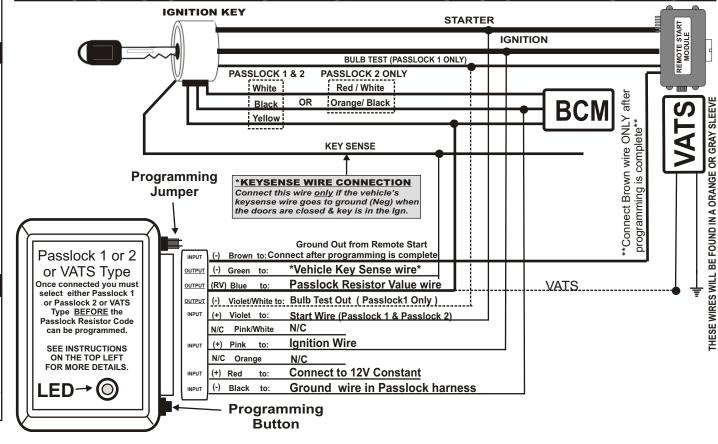
**INSTALLATION NOTES:** \*The wiring of some older model Passlock 1 may also have the following color sequence: Black/White, Black (GND), Black (DATA) \*\* The Equinox is a PASSLOCK 2 type even though it does not have a starter wire.
