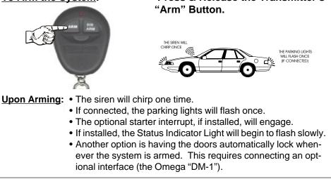
In addition to detecting impacts to the vehicle and detecting a current draw from the battery (example- interior light illuminating from opened door), the Freedom-400 has a detection circuit which may be used to protect the hood, trunk or doors. If this circuit is in a violated state when arming the system, the confirmation will be three chirps instead of one. The system will still arm, but it will bypass the open zone until the zone is secured; once secured, this zone is protected.
