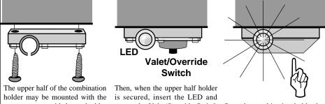
The upper half of the combination holder may be mounted with the two screws provided, or, doublesided adhesive tape may be used. Then, when the upper half holder is secured, insert the LED and mount the Valet/Override Switch using its double-sided adhesive tape.
