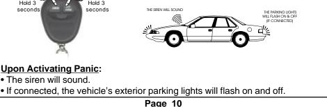
Remote Panic can be activated anytime, whether the vehicle's ignition is turned on or off, and has a 60 second duration (regardless of the 30 or 60 second activation setting) unless a transmitter is used to stop it. At the end of the 60 second cycle, the system will reset and be in either the armed state (if Remote Panic was activated by the "Arm" button) or in the disarmed state (if Remote Panic was activated by "Disarm").
