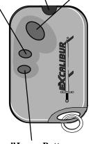
Large Upper Button-Pressing and releasing this button will arm and disarm the security system. If the optional doorlock interface is installed, the doors will lock upon arming, and unlock upon disarming.
