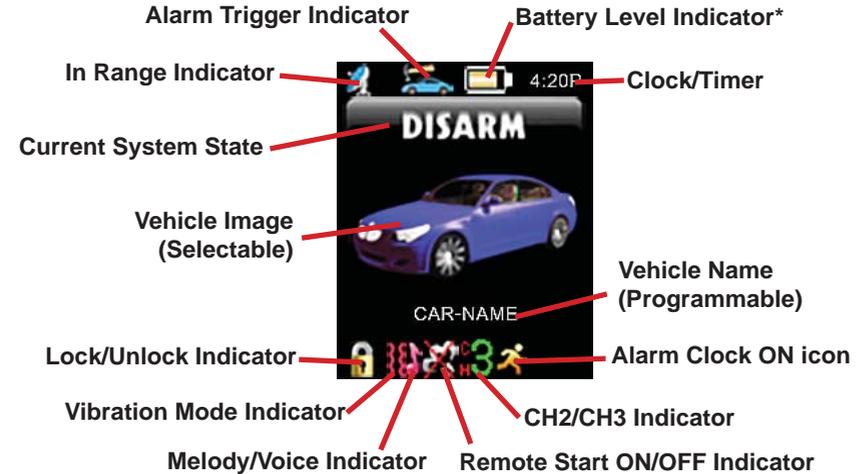
\*The controller is powered by a built-in rechargeable battery. When the battery level indicator shows a low battery, plug the supplied USB cable into the controller, then connect the other end to the supplied AC adapter or your computer's USB port. While charging, the indicator will increment from empty to full. When full, the indicator will show a plug icon.
