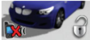
When Power Save mode is ON, you will not receive any 2-way confirmations. Additionally, there will be a red X over the “in range” indicator in the lower left corner of the status screen (pictured to the left).
