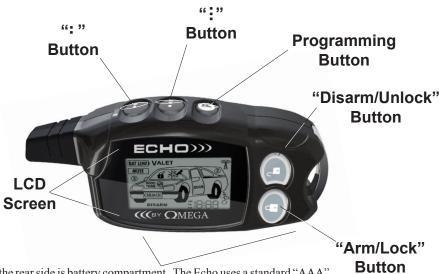
On the rear side is battery compartment. The Echo uses a standard "AAA" 1.5 volt battery, and it will indicate when to replace the battery. To replace the battery, slightly lift up on the end of the cover (there is a small indention), then slide the cover towards the bottom of the controller.
