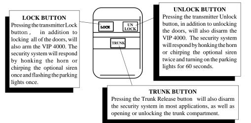
These are the the typical functions of the factory keyless entry transmitter when operating the security system. Please remember that the VIP 4000 is a universal add-on security system for existing keyless entry systems, the exact operations of the VIP 4000 are determined in some extent to the particular vehicle and/or keyless entry system.
