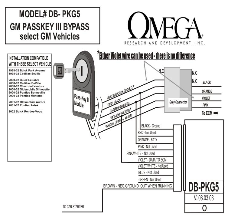
When the DB-PKG5 is correctly installed, turn the ignition key to the "ON" position for about 5 seconde, the DB-PKG5 is now programmed. Turn to the "OFF" position, then start engine with remote starter.
