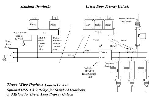
each door, which would remotely unlock all of the vehicle's doors when the K9-CLASSIC-E is disarmed. All of the added actuators would simply be wired in parallel.
