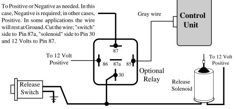
Wiring an optional Relay for Trunk Release.
