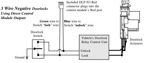
The included DLP-N3 harness can allow direct connection of the security system to the "lock" and "unlock" wires of the 3 Wire Negative Pulse system. Some doorlock systems, however, require more than the 500mA ground output that the security system's control module can accommodate. In these **Page - 23**
