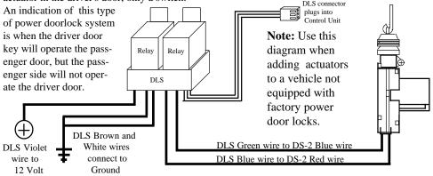
Vehicles Not Equipped With Power Doorlocks: This same type of interface can be used, with two variations: as shown, thus remotely unlocking the driver's door only, or with a DS-2 actuator in Page - 29
