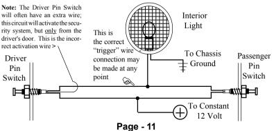
The correct wire for a Positive switching type of dome light/door jamb pin switch system will have 12 volts present when the doors are opened, and chassis ground when the doors are closed.
