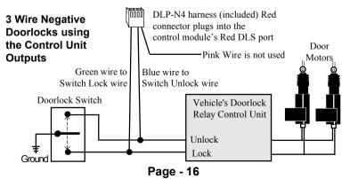
The two later wires are both routed to the doorlock actuators and are connected to either end of the actuator's motor winding. When the switch is pushed to one position, one of these two wires will have 12 volts. This voltage flows through the wire to the actuator's motor winding, and since the other wire is still <u>resting at</u> <u>ground</u> an electrical circuit is completed. When the switch is pushed to the opposite position the electrical flow is <u>reversed</u>.
