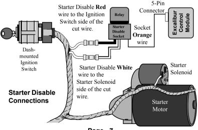
The starter wire must be located and cut. Cutting the vehicle's starter wire will result in two sides- the "ignition switch" side and the "starter solenoid" side. It is recommended that this connection be done as close to the ignition switch as possible. Use a Digital Multimeter (DMM) to find the correct wire.
