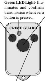
Small Right Transmitter Button- If this button is pressed and held for 3 seconds, the security system will activate the trunk release function.
