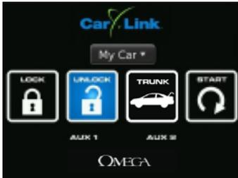
Buttons flash BLUE when activated, GREEN to confirm operation or RED to indicate the vehicle did not receive the command.
