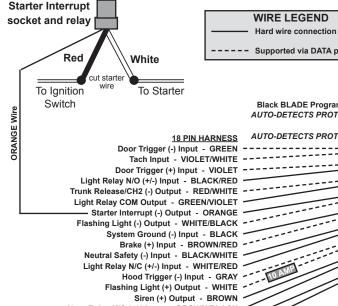
Horn Relay N/C (+/-) Input - BROWN/BLACK Horn Relay COM Output - BLUE/BLACK Horn Relay N/O (+/-) Input - VIOLET/BLACK \* Supported via DATA port(s)
