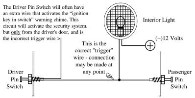
**CONNECTION:** Connect the Green wire to a wire in the vehicle that is common to all the door pin switches; the correct wire in this type of interior or dome light/door jamb pin switch system will have no voltage present and will also show chassis ground when the doors are opened, and up to 12 volts when the doors are closed.
