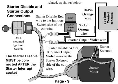
Connect the 18-pin connector's Orange wire to the Orange wire of the starter interrupt relay socket. Then make the connections which interrupt the vehicle's starter circuit- the starter wire must be located and cut. Cutting the vehicle's starter wire will result in two sides- the "ignition switch" side and the "starter solenoid" side. It is recommended that this connection be done as close to the ignition switch as possible. Use a Digital Multimeter (DMM) to find the correct wire.
