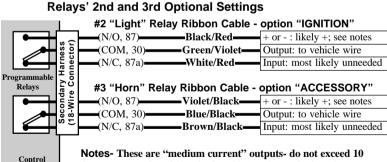
Notes- These are "medium current" outputs- do not exceed 10 Amps current draw! Use the four 30 Amp internal relays (large 6-wire connector) for traditional high-amperage ignition switch circuits.
