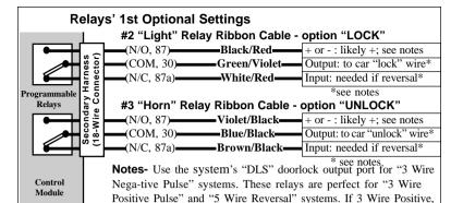
connect both relay N/O wires to Positive; relay N/C wires are not used. If 5 Wire Reversal system, connect both N/O wires to Positive; connect relay N/C wires to the doorlock switch side, connect relay COM to the actuators side. See the section "Power Doorlock Interface Port", explaining the DLS port operation, for more doorlocking system information.
