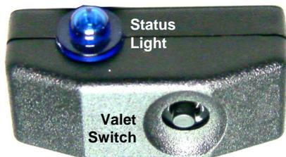
vehicle. If the optional Echo 2-way controller is used, the Status Light and Valet Switch are within a long-range receiver module, typically mounted to the windshield or other glass. The Status Light may be either blue or red; included with your Excalibur system is a blue light (red is available optionally), and it is red in the Echo receiver module.
