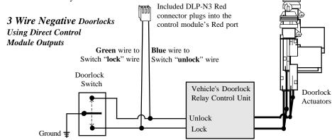
The included DLP-N3 harness can allow direct connection of the security system to the "lock" and "unlock" wires of the 3 Wire Negative Pulse system. Some doorlock systems, however, require more than the 500mA ground output that the security system's control module can accommodate. In these
