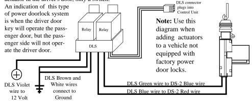
**Vehicles Not Equipped With Power Doorlocks:** This same type of interface can be used, with two variations: as shown, thus remotely unlocking the driver's door only, or with a DS-2 actuator in
