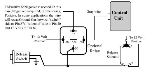
Wiring an optional Relay for Trunk Release.
