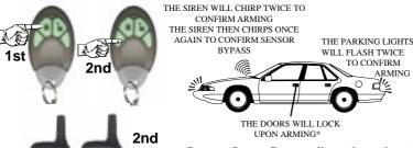
Remote Sensor Bypass allows the option of turning off" the sensor any- time the system is armed using the transmitter or transceiver. When the sensor is bypassed, only the sensor zone is bypassed and all other protected zones will remain fully operational and vigilant. The sensor zone will reset to its normal operation the next time the system is armed.
