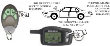
With Driver's Door Priority, again Press & Release the "Disarm/Unlock" Button ( 1) to unlock the remaining doors
