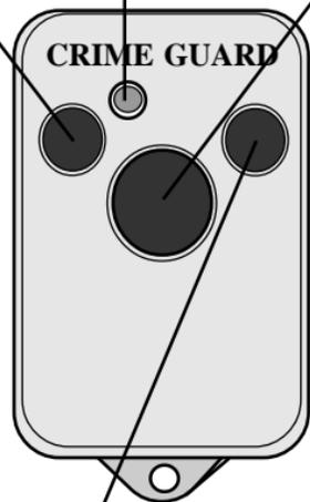
**Small Right Transmitter Button-** If this button is pressed and held for 3 seconds, the security system will activate the trunk release function.
