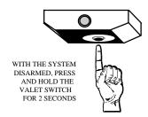
The Valet Switch is in the Status Indicator Light/Valet Switch Assembly. The installer has the option of utilizing an additional, separate Valet Switch should mounting in a hidden location be desired. Please become familiar with the location of the Easy Valet switch.
