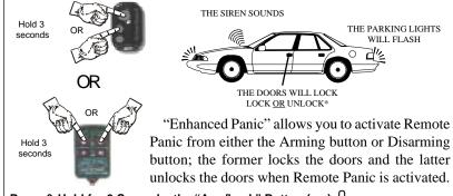
Press & Hold for 3 Seconds the "Arm/Lock" Button ( ) OR the "Disarm/Unlock" Button ( Optional 4 Button Transmitter
